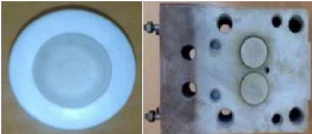
Figure 2. PSZ coated piston and valves
