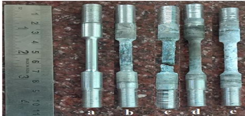
Fig 9 Photographs of SCC test on different AA 7xxx + 0.5 % SC alloy a) Cast b) Cast after SCC c) Solutionized (450°C-24hrs) after SCC d) Aged (120°C-20hrs) after SCC and e) Aged (160°C-20hrs) after SCC.
