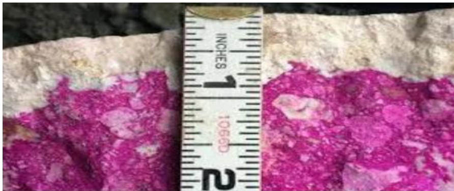
Fig. 17. Measurement of Carbonation Depth in the concrete sample.
