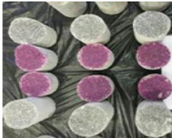
Figure 9 : Carbonation Test for SCBA
