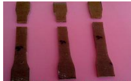
Fig. 2(b)-G/H/F Tensile after Testing
