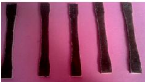
Fig. 2(a)-G/H/F Tensile Specimen
