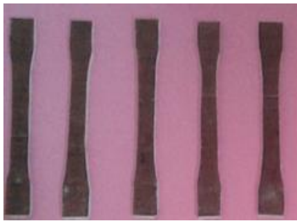
Fig. 2(a)-G/J Tensile Specimen
