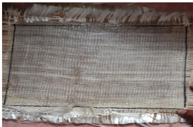
Figures 1 Composite material by hand layup method.
