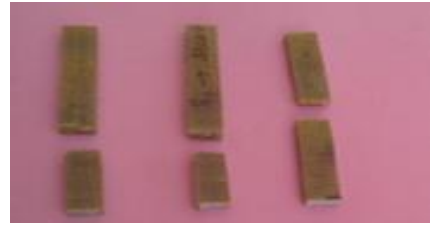
Fig-3(b)-G/C-flexural after testing
