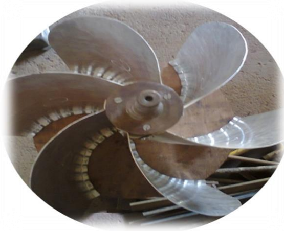
Figure 3: Finalized Modified Turbine Model
