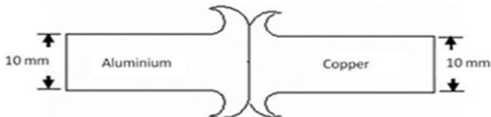
Fig. 2. Typical weld design and assembly for friction welding
