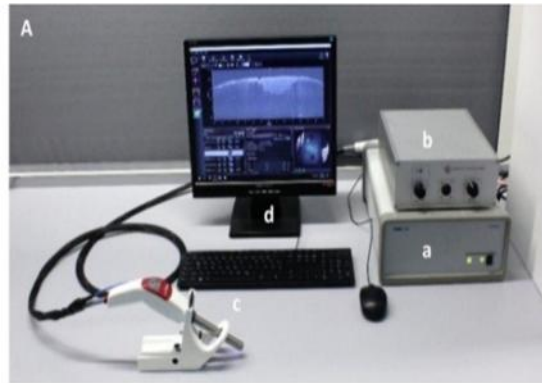
Figure 1: Photograph of a OCT system setup (a) Scanner controller (b) balance detector (c) OCT probe (d) computer
